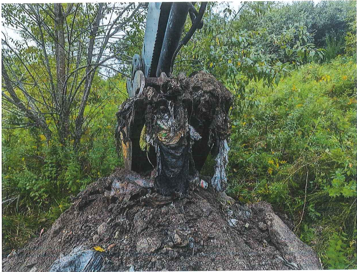
Photo 28: TP23-18 close up of excavated waste material
